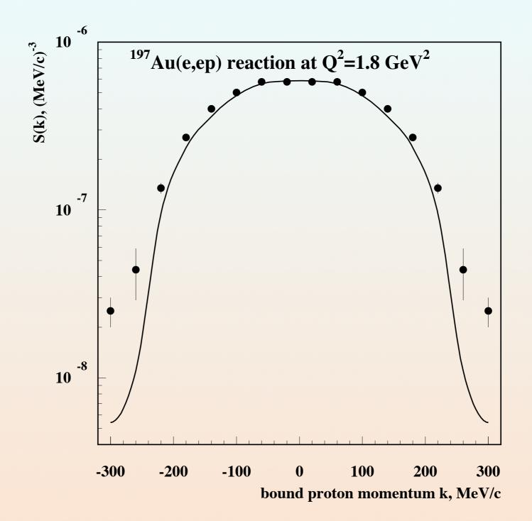
Eikonal approximation usually neglects change of the transverse nucleon momentum in the final state rescatterings.We checked that account of this effect leads to a small correction for k<200 MeV/c
