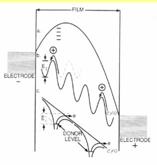
**Figure 10-8.** Bulk-limited conduction mechanisms. (Dotted lines refer to  $\mathscr{E} = 0$ ) (a space-charge-limited; (b) ionic conduction of cations  $\oplus$ ; (c) Poole-Frenkel.
