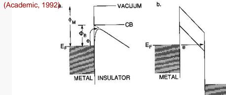
Figure 10-7. Barrier limited conduction mechanisms. (a) Schottky emission; (b) tunneling.
