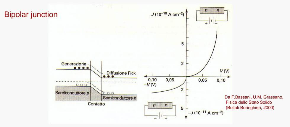
In the absence of an applied field, p and n charges are redistributed so to create a junction (a charge-free region similar to a capacitor)
