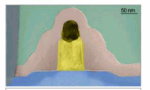
**One in 58 Million.** A transistor just 90nm wide (yellow) on substrate of SOI (blue) with copper interconnects (gray). Layers of nitride (brown) and oxide (green) insulate it from its brethren. Magnified 146,000 times.
