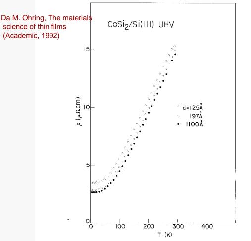
**Figure 10-6.** Temperature dependence of resistivity of  $CoSi_2$  films. The 125-Å and 197-Å films are epitaxial. The 1100-Å film is polycrystalline. (From Ref. 10).
