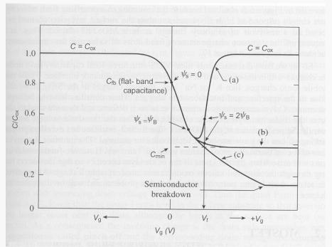
Figure 6: C-V curve of an ideal MOS capacitor under
