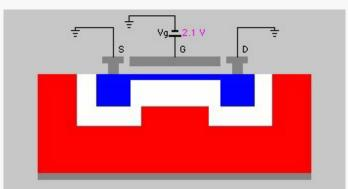
Enhancement-mode (Normally-off) MOSFET N-channel Vg > Vt: gate bias is more positive than the threshold voltage. Sufficient electrons accumulate and forms the inversion channel.
