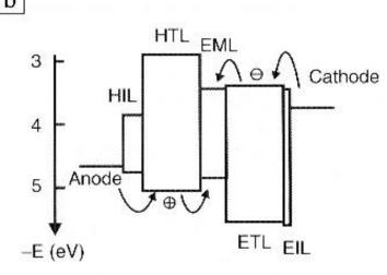
Figure 2. (a) Structure and (b) energy-level diagram of a typical organic light-emitting diode (OLED).
