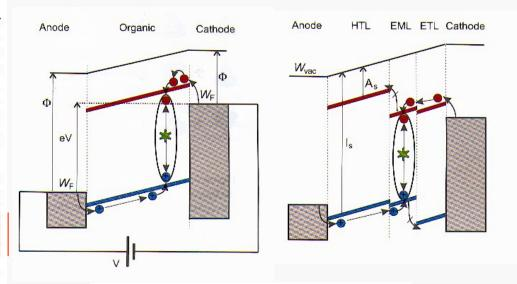
Figure 5: Energy level scheme for a single layer (top) and double heterojunction OLED (bottom) with an applied bias voltage V showing the vacuum energy level  $W_{\text{vac}}$ , the Fermi levels  $W_{\text{F}}$  and workfunctions  $\Phi$  of the metallic contacts and the hole and electron transport levels of the organic layers. The level offsets at the organic heterojunctions are determined by the different ionization energies  $I_s$  and electron affinities  $A_s$  of the adjacent layers.
