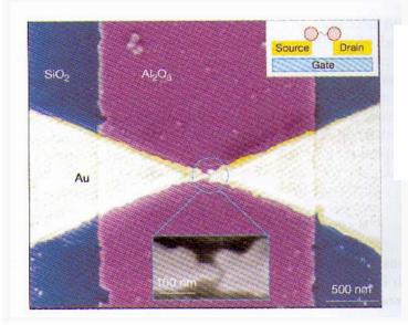
Figure 9: SEM picture of a Au electrode pair on top of an Al gate electrode, which is covered by an Al<sub>2</sub>O<sub>3</sub> insulator. Such a setup was used as a molecular field effect transistor [47].
