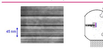
Cross-section of a few stages of QC-laser crystal crystal growth one atomic layer at a time
