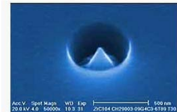
This carbide crystalline tip, with a radius of 100 angstroms, or 10 nanometers at the top and 0.5 micron at the base, emits electrons in a tiny beam.
