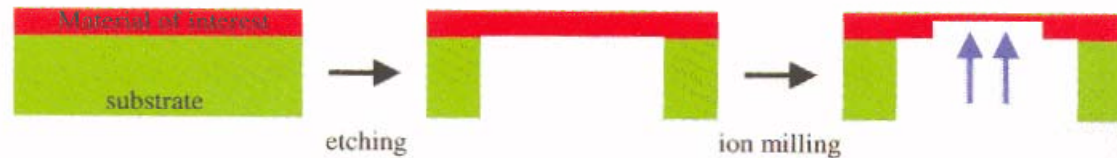
Figure 16: Schematic procedure to prepare a planar sample for TEM. After preparing the sample on an substrate the latter may be etched. The final thickness of some 100 nm can be achieved by ion milling. The up pointing arrows denote the direction of the TEM beam.
