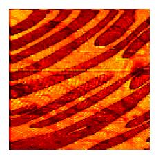
Image of ferroelectric domain structure in TGS Sample by Voltage Modulation Atomic Force Microscopy Scan size 27 μm x27 μm
