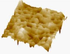
The sample is a strip of adhesive (3M Scotch tape) that has been peeled of a metal surface. The image shows small pits in the sticky surfaces of the adhesive. The image was acquired in TappingMode at frequency of 3 Hz and setpoint of 1.8 V.  $2\mu m$  scan courtesy L. Scudiero, Washington State University, USA.
