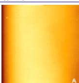
Figure 13A-B: Image (A) is an 85 X 85 micron image of a flat piece of silicon. The bow introduced into the image is seen at the edges. (B) A line profile across this image shows the magnitude of the bow. (Image) post-processing can help (but can also introduce new artifacts, as well...)
