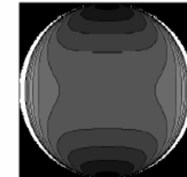
Fig. 3. Total electric field |\vec{E}|^2 in the aperture obtained by Bouwkamp.
