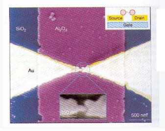
Figure 9: SEM picture of a Au electrode pair on top of an Al gate electrode, which is covered by an  $Al_2O_3$  insulator. Such a setup was used as a molecular field effect transistor [47].
