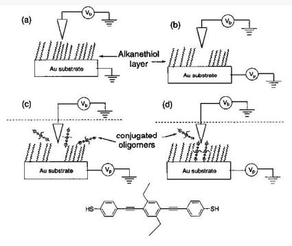
Figure 4.6 Schematic representation of the lithographic patterning and replacement c. conjugated molecules in an alkanethiolate matrix. (a) Normal STM imaging of an alkanethiolate SAM with tip bias  $V_{b}$ . (b) SAM removal by applying a voltage pulse  $V_{p}$  to the substrate. (c) Carrying out the same voltage pulse as in (b), but under a solution of molecular wires (expanded structure at bottom) causes (d) insertion of the wires into the newly vacated site.
