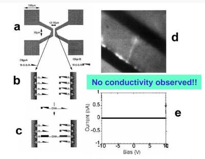
Fig. 1 a-c  $16-\mu$ m-long  $\lambda$ -DNA was stretched between two metal electrodes using short hang-over single strands complementary to single strands that were preattached to the metal electrodes. d A fluorescent image of the DNA molecule, connecting the metal electrodes. e The flat, insulating current-voltage that was measured. (from [12], with permission; Copyright 1998 by Nature Macmillan Publishers Ltd)
