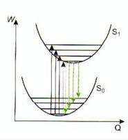
**Figure 4:** Potential energy lines and vibronic levels for the ground state  $S_0$  and the first excited state  $S_1$  as a function of a configuration coordinate Q reflecting the intramolecular atomic distances. The electronic transitions without change in Q are always most pronounced in the spectra. Clearly, the absorption wavelengths (black) are larger, in general, than the emission wavelengths (green), causing a red shift of the emission spectrum with respect to the absorption spectrum.
