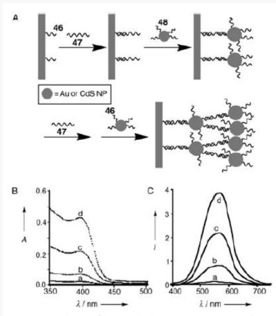
*Figure 20.* A) The use of DNA as a linker to construct nanoparticle multilayers on surfaces. B), C) The absorbance and the fluorescence spectrum, respectively, of the CdS NP multilayer assemblies: a)–d) 1 to 4 layers. (Parts B and C are adapted from Ref. [188], with permission).
