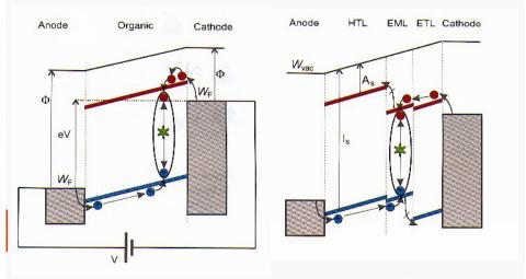
Figure 5: Energy level scheme for a single layer (top) and double heterojunction OLED (bottom) with an applied bias voltage V showing the vacuum energy level  $W_{vac}$ , the Fermi levels  $W_F$  and workfunctions  $\Phi$  of the metallic contacts and the hole and electron transport levels of the organic layers. The level offsets at the organic heterojunctions are determined by the different ionization energies  $I_s$  and electron affinities  $A_s$  of the adjacent layers.
