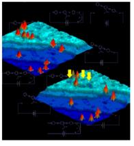
We use self-assembly to control and STM to observe the switching of single molecules.
