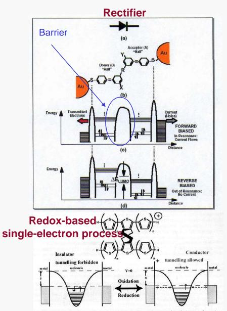
Figure 2.4:- The tranport mechanism responsible for the conduction and insulation transformation through the reduction / oxidation of a molecule. The mechanism is similar to Coulomb blockade.
