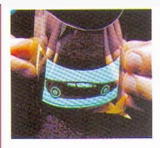
Figure 15: A flexible 0.18 mm thick passive matrix OLED display fabricated by Universal Display Corporation.
