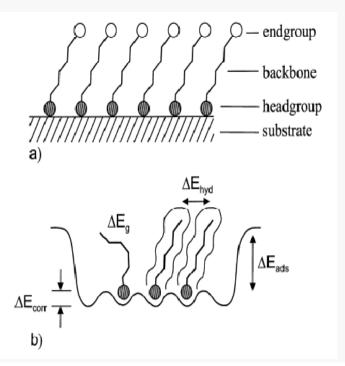
Fig. 2. (a) Schematic of SAM. Shaded circle indicates chemisorbing headgroup and open circle endgroup, which can be chosen from variety of chemical functionalities. (b) Schematic of different energies.  $\Delta E_{ads}$  stands for adsorption energy,  $\Delta E_{corr}$  corrugation of substrate potential experienced by molecule,  $\Delta E_{hyd}$  van der Waals interaction of (hydrocarbon) tails, and  $\Delta E_g$  energy of gauche defect (or, generally, deviation from fully stretched backbone).
