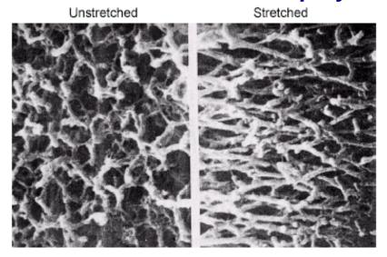
Stretching polyacetylene aligns the chains and improves conductivity. Each fiber shown here consists of about 1,500 polymer chains. <u>A goal of</u> molecular electronics is to use individual polymer chains.
