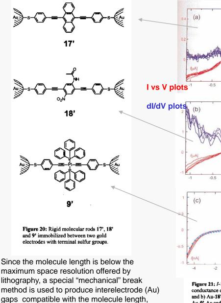
Figure 21: *I-V* curves (red) and differential conductance d*I/dV* (blue) for a) Au-17'-Au and b) Au-18'-Au. c) *I-V* curve (red) for Au-9'-Au and simulated current with a barrier height of 2.5 eV (blue circles) are shown.
