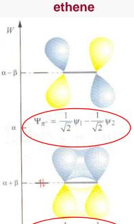
Figure 15: Result of the HMO calculation for ethene: energy levels and sketch of the wave functions of the  $\pi$ -MOs. The occupation of the energy
