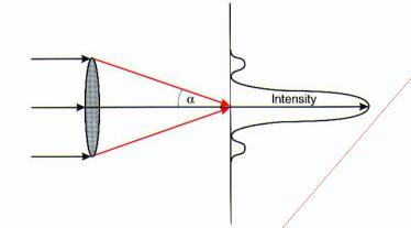
Figure 3.8 The Abbe equation gives the width of the first intensity peak for the image of point object at infinity in terms of the angular aperture of the lens  $\alpha$  and the wavelength of the radiation  $\lambda$
