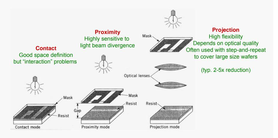
Presently: **projection** modes are most common in industrial implementations, typically implemented with "step and repeat" techniques (a small region of the substrate is impressed and then the substrate is moved to repeat the patterning over a larger area)
