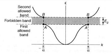
In solid-state physics: In a crystal lattice, a periodic potential leads to the appearance of energy **gap** for the electron wavefunction
