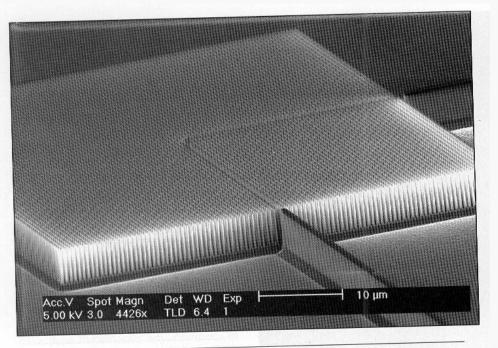
Figure 4. Scanning electron micrograph of a periodic array of silicon pillars fabricated using deep anisotropic etching. The silicon pillars are 205 nm in diameter and 5  $\mu$ m tall. This structure possesses a bandgap of around 1.5  $\mu$ m for transverse magnetic polarization. By removing an array of pillars, a waveguide bend may be fabricated. Input and output waveguides are integrated with the photonic crystal.
