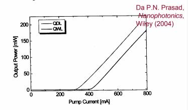
Figure 4.19. Comparison of efficiency between a quantum well laser and a quantum dot laser.
