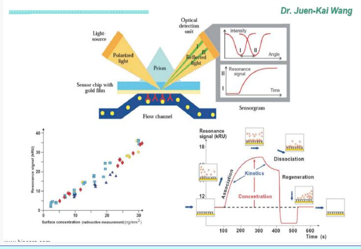
Surface plasmons are frequently exploited in a variety of applications, including highly-sensitive spectroscopy methods
