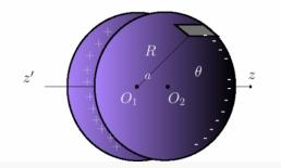
The polarization induced electric field is colinear but in the opposite direction to the external field. It is called depolarizing field.
