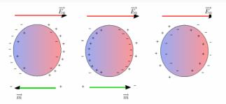
Schematics of the three different cases of polarization depending on the Clausius-Mossotti factor under an electric field. From left to right: the particle is not much polarizable before the surrounding environment; the particle is very polarizable before the surrounding environment; the particle is as polarizable as the surrounding environment.
