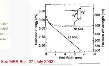
Figure 3. Transition energy of  $Ga_{0,g}in_{0,1}N/GaN$  quantum wells versus well width, with and without built-in electric field. The inset shows a schematic view of the band scheme, the effective bandgap  $E_g^{\text{eff}}$ , and the original bandgap  $E_g^{0}$ .
