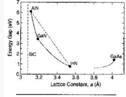
Figure 1. Fundamental bandgap versus basal-plane lattice constant of nitride materials compared with SiC and GaAs. The solid curves represent the ternary mixtures AIN/GaN,<sup>10</sup> GaN/InN,<sup>11</sup> and GaN/GaAs.<sup>12</sup> The dotted curve qualitatively indicates the continuation of the GaNAs gap toward GaN.
