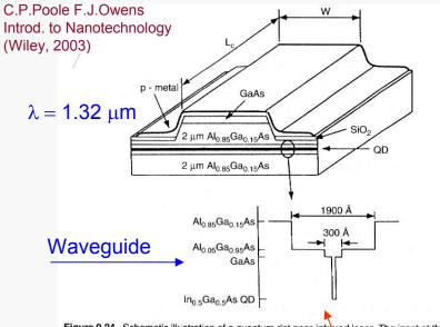
**Figure 9.24.** Schematic illustration of a quantum dot near-infrared laser. The inset at the bottom shows details of the 190-nm-wide ( $Al_{0.85}Ga_{0.15}As$  cladded) waveguide region that contains the 12 monolayers of  $In_{0.5}Ga_{0.5}As$  quantum dots (indicated by QD) that do the lasing. [From Park et al. (1999).]
