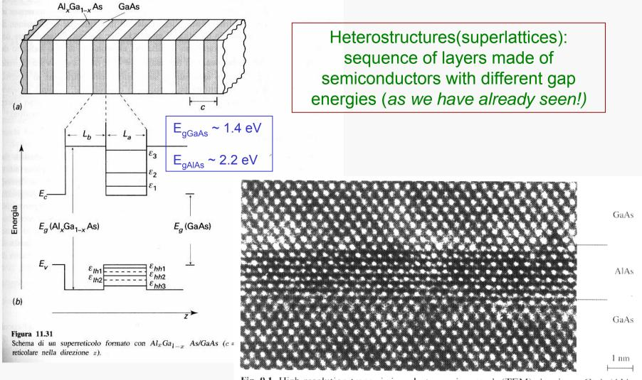
Da Bassani Grassano, Fisica dello Stato Solido, Boringhieri (2000) **Fig. 9.1.** High resolution transmission electron micrograph (TEM) showing a GaAs/AlAs superlattice for a [110] incident beam. (Courtesy of K. Ploog, Paul Drude Institute, Berlin.) In spite of the almost perfect interfaces, try to identify possible Al atoms in Ga sites and vice versa
