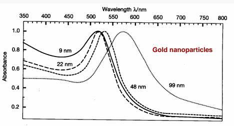
Figure 5.1. Optical absorption spectra of gold nanoparticles of different sizes. From Link and El-Sayed (1999), reproduced with permission.
