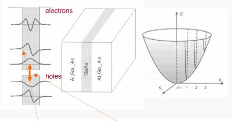
• For energies E < V, the energy levels of the electron are quantized for the direction z of the confinement; hence they are given by the model of particle in a one-dimensional box. The electronic energies in the other two dimensions (x and y) are not discrete and are given by the effective mass approximation discussed in Chapter 2. Therefore, for E < V, the energy of an electron in the conduction band is given as
