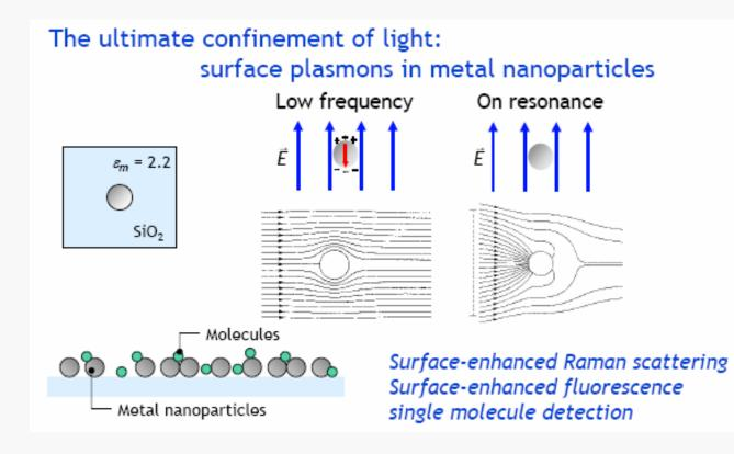
Surface plasmon nanophotonics: optics below the diffraction limit
