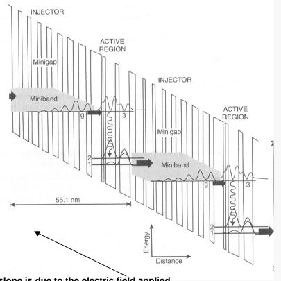
The slope is due to the electric field applied
