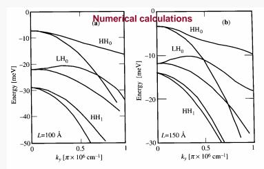
**Fig. 9.6.** Hole subband energies in a GaAs/Ga<sub>0.7</sub>Al<sub>0.3</sub>As QW calculated by *Bastard* and *Brum* [9.18] within the envelope-function approximation for well widths of (**a**) 100 and (**b**) 150 Å, respectively. The labels HH and LH denote the subbands arising from the heavy and light hole valence bands in the bulk, respectively (*red curves*). The *black curves* represent the subband energies calculated when the mixing between the heavy and light hole bands is neglected
