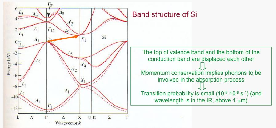
Fig. 2.10. Electronic band structure of Si calculated by the pseudopotential technique. The *solid* and the *doted lines* represent calculations with a **nonlocal** and a **local pseudopoten**tial, respectively. [Ref. 2.6, p. 81]
