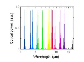
QC lasers cover entire mid-infrared wavelength range  $(3.4 - 17 \ \mu m)$  by tailoring layer thicknesses of the same material
