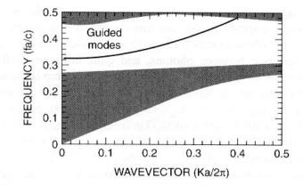
**Figure 6.32.** Effect of removing one row of rods from a square lattice of a photonic crystal, which introduces a level (guided mode) in the forbidden gap. The ordinate scale is the frequency f multiplied by the lattice parameter a divided by the speed of light c. [Adapted from J. D. Joannopoulos, *Nature* **386**, 143 (1997).]
