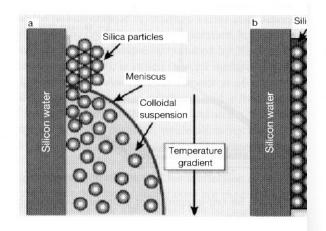
Figure 9.13. Vertical deposition method for crystallization of colloid duced with permission from Joannopoulos, J. D., *Nature* 414, 257–258 (2)
