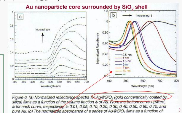
Color depends on particle size, features of the sorrounding dielectric and interparticle spacing (collective interparticle effects!)
