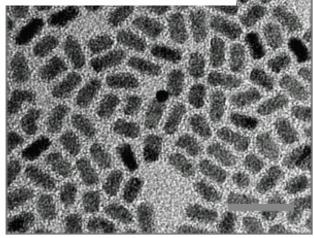
**Electron Micrograph.** Transmission electron microscopy can be used to directly image Qdot core-shell nanocrystals. The darker regions are the crystallites. Like several of QDC's products, these core-shell nanocrystals are rod-like in structure. The magnification is 200,000 and the scale bar is 20 nm.
