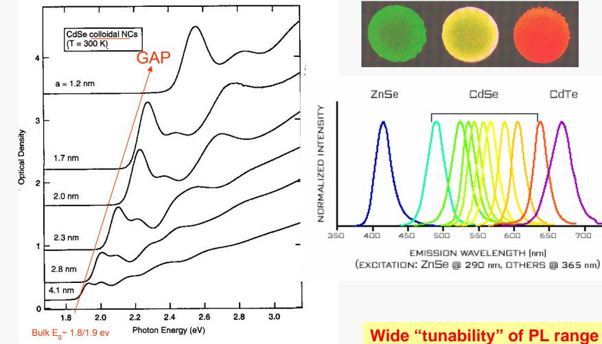
jure 3.27. Room-temperature optical absorption spectra for CdSe colloidal nanocrystals Cs) with mean radii in the range from 1.2 to 4.1 nm. [From V. I. Klimov, in Nalwa (2000), I. 4, Chapter 7, p. 464.]
