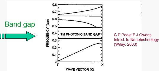
A simple 2D PC (reg. array of dielectric cylinders)
