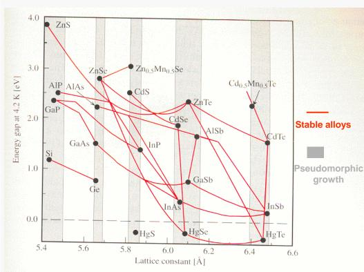
Fig. 9.2. A plot of the low temperature energy bandgaps of a number of semiconductors with the diamond and zinc-blende structure versus their lattice constants. The *shaded regions* highlight several families of semiconductors with similar lattice constants. Semiconductors joined by *solid lines* form stable alloys. [Chen A.B., Sher A.: *Semiconductor Alloys* (Plenum, New York 1995) Plate 1]
