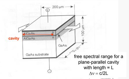
Figure 4.17. Scheme of double heterostructure semiconductor (DHS) lase
