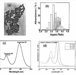
FIGURE 3. (a) TEM image of gold nanorods synthesized electrochemically in micellar solution<sup>38</sup> under the best conditions. (b) Size distribution of the nanorods. (c) Absorption spectrum of these nanorods. (d) Simulated spectra of nanorods of different aspect (length to width) ratios.
