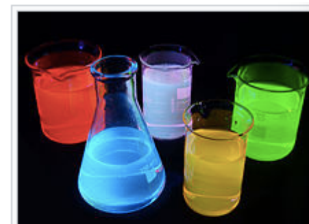
Fluorescence of different substances under UV light. Green is a fluorescein, red is Rhodamine B, yellow is Rhodamine 6G, blue is quinine, purple is a mixture of quinine and rhodamine 6g. Solutions are about 0.001% concentration in water.
