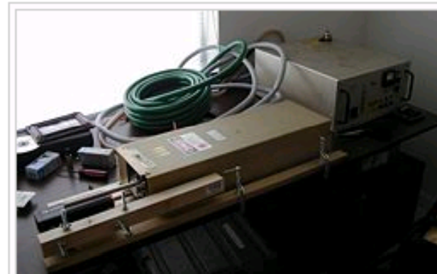
From left to right: 1 mW Uniphase HeNe on alignment-rig, 2 Watt Lixel 88 Argon Ion laser, and power-supply. To the rear are hoses for water cooling.
