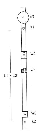
Figure 1: Diagram of the Kater pendulum. The symbols  $L_1$  and  $L_2$  on the figure are  $\ell_1$  and  $\ell_2$  in the text.  $L = \ell_1 + \ell_2$  is the distance between fulcrum points. The distances of most of the weights from each fulcrum are adjustable. Note that W2 is between W4 and W3, rather than as shown.
