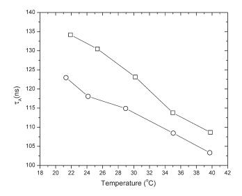
**FIGURE 7** Acoustic damping time versus temperature for PMMA ( $M_w = 120,000$ , circle) and PMMA ( $M_w = 996,000$ , square).
