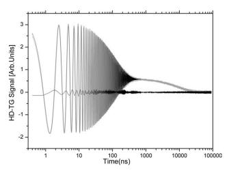
**FIGURE 2** HD-TG data (gray line), fit (black line), and residues (lower lines) for PMMA ( $M_w = 120,000$ ), at the T = 24 °C and at wave-vector  $q = 1 \ \mu m^{-1}$ .
