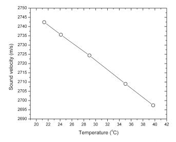
**FIGURE 3** Sound velocity versus temperature for PMMA ( $M_w = 120,000$ ).
