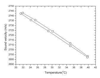
**FIGURE 6** Sound velocity versus temperature for PMMA ( $M_w = 120,000$ , circle) and PMMA ( $M_w = 996,000$ , square).
