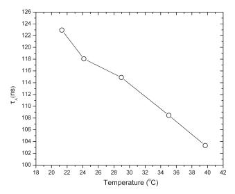
**FIGURE 4**  $\tau_A$  versus temperature for PMMA with  $M_w = 120,000$ .
