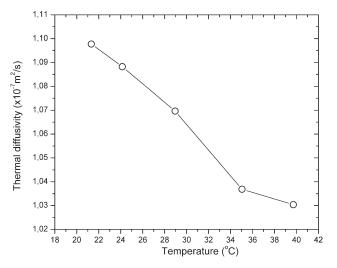
**FIGURE 5** Thermal diffusivity versus temperature for PMMA ( $M_w = 120,000$ ).
