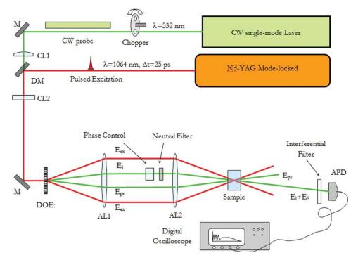
**FIGURE 1** Optical set-up for a HD-TG experiment, CL, cylindrical lens; M, mirror; DM, dichroic mirror; DOE, diffractive optic element; AL, achromatic lens; ADP, avalanche photodiode;  $E_{l}$ , local field;  $E_{pr}$  probe field; and  $E_{ex}$  is excitation field.
