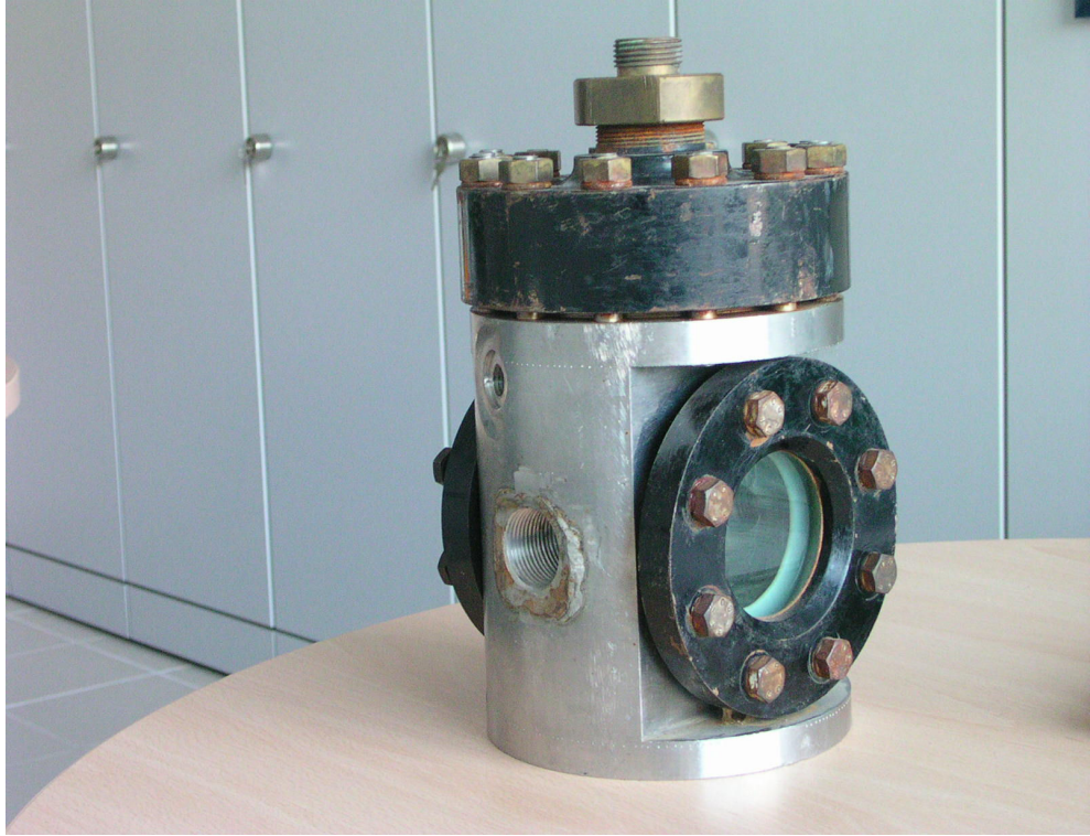
Figure 8: One of the earliest prototype bubble chambers
