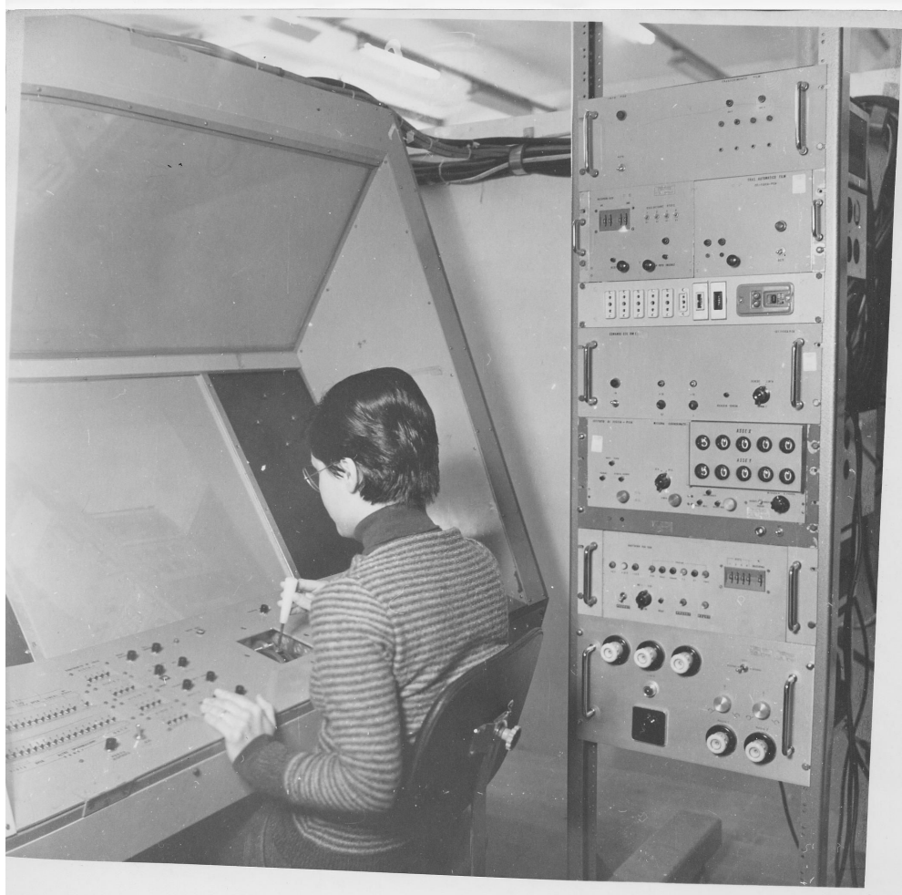
Figure 28: Patrizia Benfatti at work on a precision manual measuring machine
