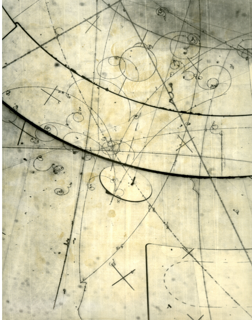
Figure 43: A neutrino interaction in BEBC filled with Neon-Hydrogen: search for neutrino oscillations in the PS180 Experiment
