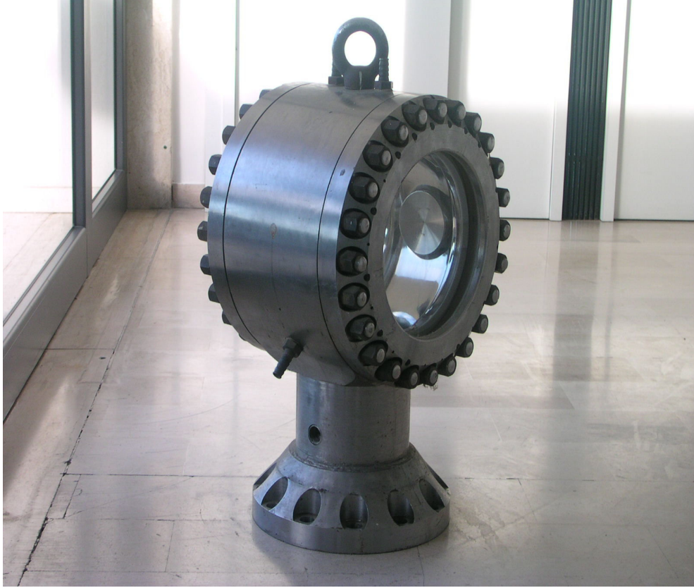
Figure 11: The body of the propane bubble chamber
